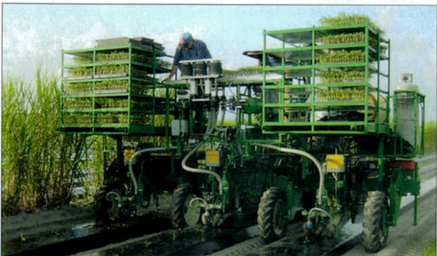
Renaldo's RTMA automatic transplanter uses propane to burn a hole in the plastic mulch that covers row crops (top left) to transplant seedlings or plant seeds.
