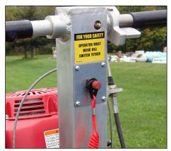
unit, falls, or becomes disabled in any way the kill switch is activated stopping the unit in its tracks. A thumb control on the handle bar allows the operator to control the direction of the unit without ever removing his hands from the steering handle, allowing for greater safety and control of the dolly.
