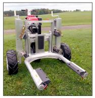
Gone is the conventional transmission and dual drive wheels. This is 100% hydraulic drive. The HONDA® GXV390 13 HP OHV, gasoline engine provides ample power to the pump. A tethered kill switch, which attaches to the operators wrist, provides an added measure of safety. If operator looses control of the
