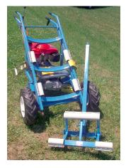
The RTC120 adapter is designed to carry a single 120 gallon, horizontal style propane storage tank. This kit includes the adapter, strap, ratchet modifications and installation and operating instructions. This is NOT capable of handling 250 gallon ASME tanks. This adapter makes the handling of these tanks a one or two man operation.
