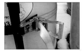
7. Using both hands, grip the handle bars and pull the unit down into position for transporting.
