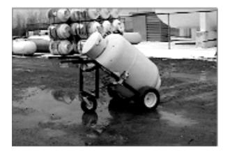
**Notice:** A cylinder should never come in contact with metal. Occasionally check the rubber pads and nylon straps for any wear.
