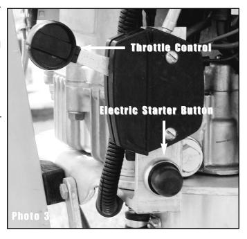
F. To shut down the engine, move the throttle control lever to the off position, or release the handle.
