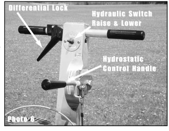
D. Returning the handle to the neutral position slows the unit, and once the detent is reached the tank carrier will come to a complete stop. In the detent position the drive wheel is locked. The same condition occurs when the engine is not running, regardless of the position of the handle.
