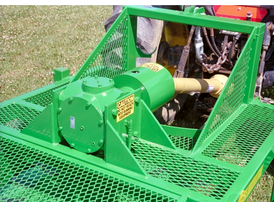
100 HP Bondioli & Pavesi Gear Box and Drive Line.
