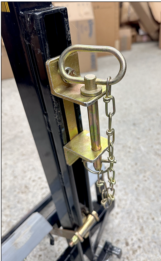
Top Yoke w/ Hitch Pin. Loosen hex head bolt to adjust accordingly.
