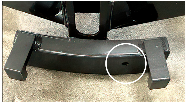
Position of Pre-Drilled Hole. Insert clevis pin through bottom cross brace and pre-drilled hole to secure to dolly.
